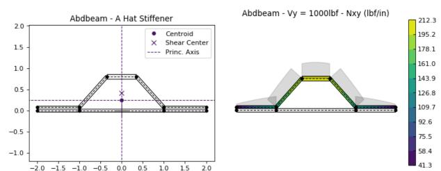
Abdbeam is a python package for the cross section analysis of thin-walled composite material beams of any shape.
