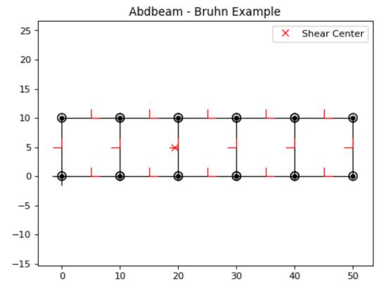
Next we'll create the load case, calculate its internal loads and obtain the shear flows accessing the internal loads Pandas dataframe sc.sgs\_int\_lds\_df directly. Since the segments develop no bending resistance, the shear flow between adjacent points will be constant, and the average Nxy per segment is appropriate:
